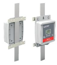
ProLEC Basic is a basic lightning current sensor that detects and logs lightning discharges flowing through the down-conductor. It is capable of measuring and withstanding currents up to 100 kA (10/350 μs).
