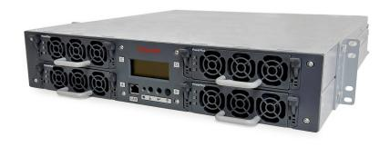
The PowerPlus System is a power conversion system for up to 12 independent high power DC circuits, with a maximum load current of 50A each, feeding new generation-high power RRH units.
